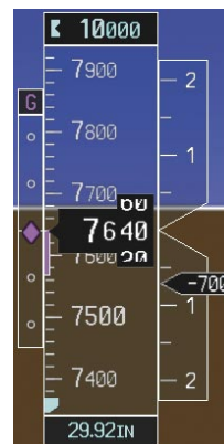
Figure 7-47 Descending to the Missed Approach Point
